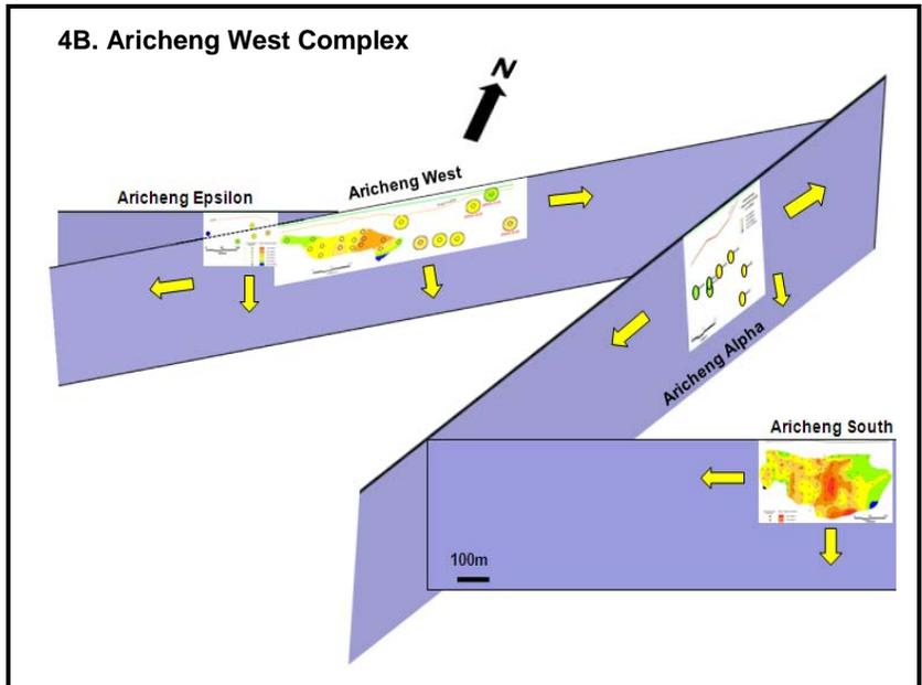
**4B.** The Aricheng West Complex consists of a northeast-trending shear zone that contains uranium at Aricheng Alpha, and two east-trending faults containing mineralization in the Aricheng West and Aricheng South sectors of those structures. The uranium-bearing zone at Aricheng Epsilon is believed to be part of the Aricheng West fault.
