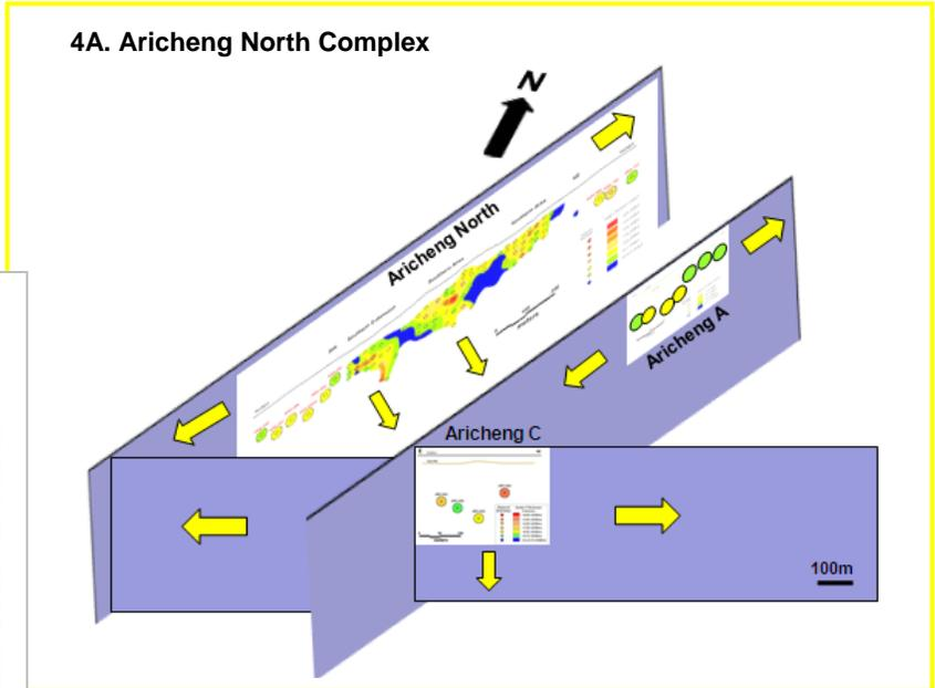
**4A.** The Aricheng North Complex consists of two northeast-trending shear zones and an east-trending fault. The northeast-trending shear zones contain uranium in the Aricheng North and Aricheng A areas and mineralization at Aricheng C (assay results reported in this press release) is located within the east-trending fault.
