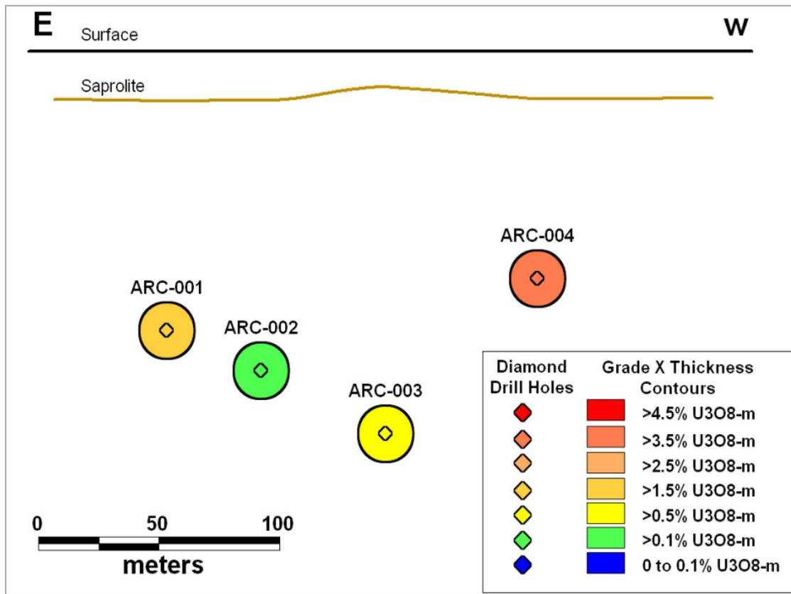
A provisional long section of the Aricheng C structure shows the distribution of grade-thickness values (the product of the width of the mineralized interval and its U<sub>3</sub>O<sub>8</sub> grade in %) on a vertical projection of the structure. A pierce point is the approximate location at which each bore hole intersects the mineralization.
