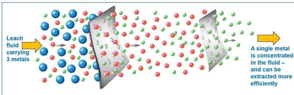
**Figure 1. Illustration of membrane screening technology to concentrate molecules of interest for recovery from the pregnant liquor solution derived from extracting commodities from mineralized rock.**
